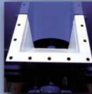
Integral feed chute directs material into center of counter rotating cages.
